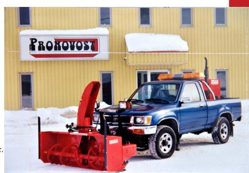
Old model of an hydraulic snowblower on a pickup truck.
